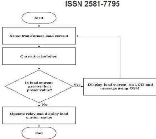
Figure 2 Flowchart for transformer load conditions
