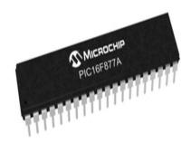
Figure 4 Microcontroller PIC16F877A
