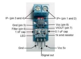
Figure 5 Current sensor (ACS712-20A module)
